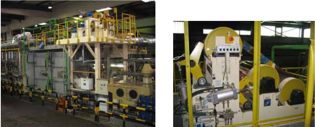
Figure 6: WSP floatation furnace and special 3 roll bridge above the water lute in already existing strip line upgraded for thin strips at Diehl Metall Sundwiger Messingwerke GmbH & Co. KG, Germany
