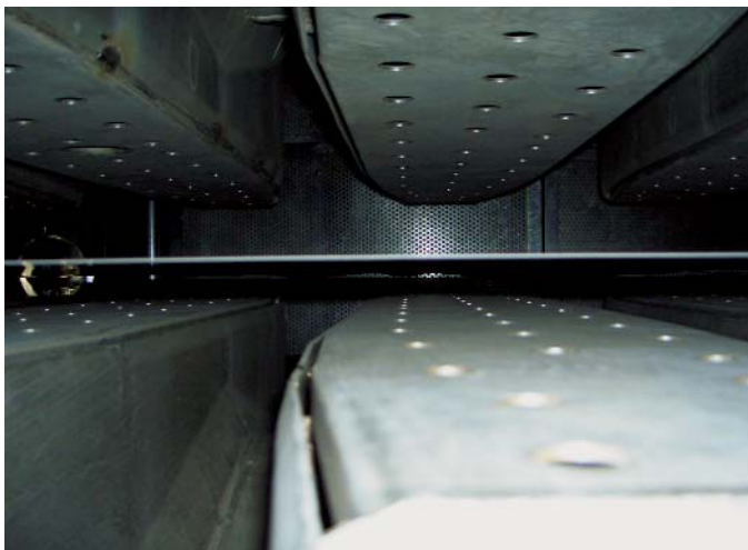
Fig. 4: Strip floating in a cooling plant of a cold strip line
